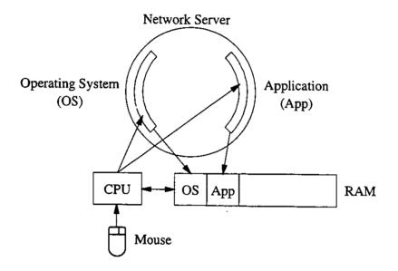
Several simplified steps in the process of starting up the computer and loading an application are represented by the numbers below:
